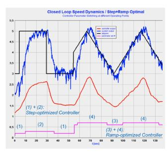
RPM Control of an engine which is difficult to control due to nonlinearities and strong noise.
